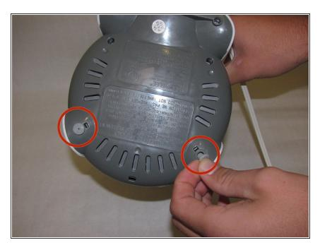
Facing the bottom of the TF6, carefully pull the two rubber feet out with your hands.
