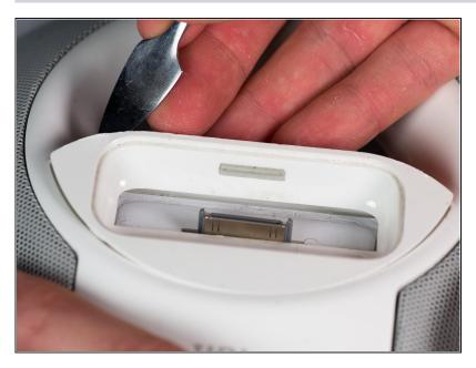
• Use a metal spudger to pry out the plastic surrounding the 30pin connector.
