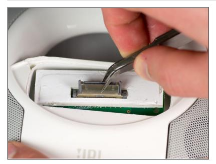
• Use a pair of <u>tweezers</u> to wiggle out the 30-pin connector.
