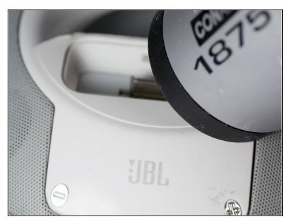
• Apply heat with a heatgun on a low setting to the area around the 30-pin connector until you can easily pry it out by the seam surrounding it (about 10 minutes).
