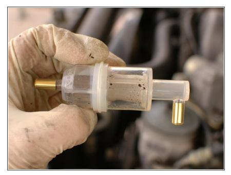
• Here is the old primary filter, removed from the car. Note the large chunks of debris in the filter.
