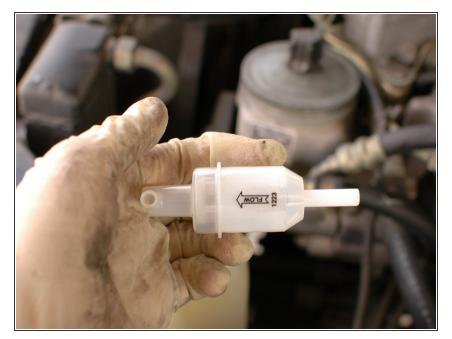
• You can see here the new primary filter. Note that the filter is usually marked with an arrow noting the direction of fuel flow. It should be installed with this arrow pointing towards the engine.
