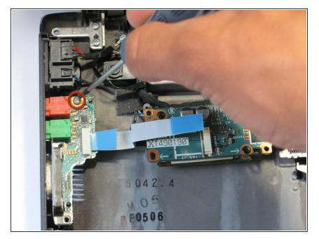
• Remove the screws for the second ethernet circuit board.
