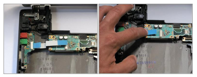
• Remove the blue ribbon from the Ethernet Circuit Board.
