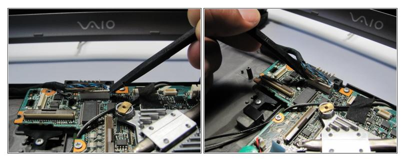
• Remove the LCD display ribbon with a nylon spudger.
