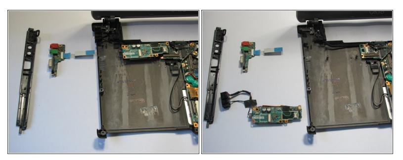
• Remove the ethernet ports.
