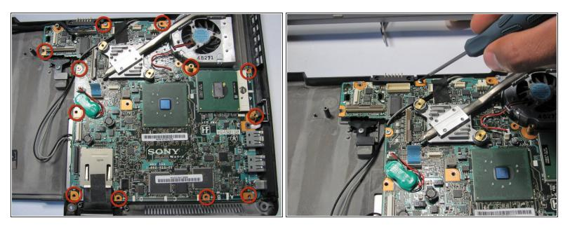
Remove screws on the motherboard.
