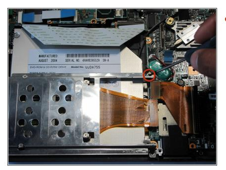
Remove the screw holding the optical drive casing to the logic board.
