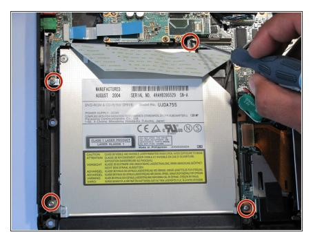
• Remove the four screws holding the optical drive to the logic board.
