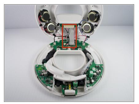
Disconnect the ribbon cable connector from the top half of the device by pulling outward and parallel to the connecting pins.
