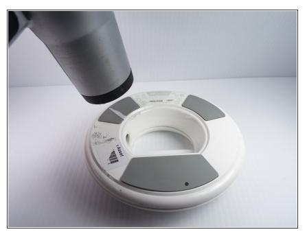
Use a heat gun (set to low) to apply heat to one of the rubber pads until you can easily remove the pad. This step takes around 5-7 minutes.
