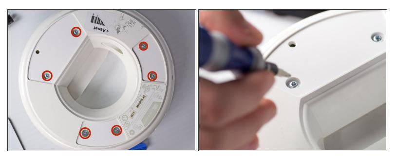
Remove the six 1cm T-10 torx screws on the bottom of the device (found under the rubber pads) using a T-10 Torx screwdriver.
