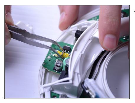
Remove the metal U-clip (compressing the spring) with tweezers.
