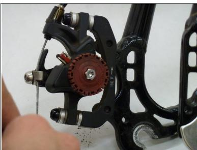
Screw the brake pad cap back on.
