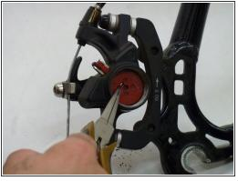
Push the spring back into place between the two brake pads so the spring is visible in the hole shown here.
