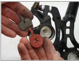
Slide out the back brake pad first. Then slide out the front brake pad.
