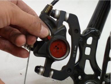
Slide in the new brake pads with the first going in the front.
