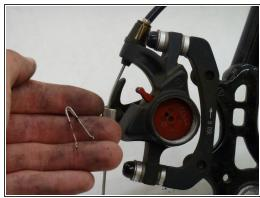
Grab and pull out the spring between the brake pads.
