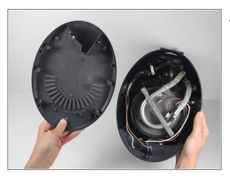
Gently lift the base cover to expose the inside of the coffee machine.
