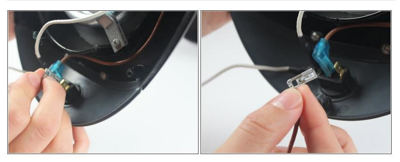
Grasp the copper cord close to the power switch. Lightly pull the silver end tab from the end to detach it.
