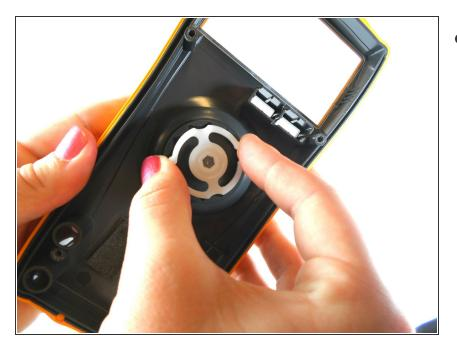
• With the dial loosened, pull the white plastic rotating piece until it comes off the dial axle.
