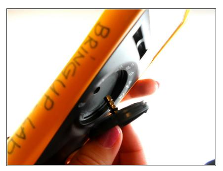
• Finally, push again on the dial axle with your thumb while at the same time pulling the dial off the front panel with your other hand .
