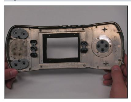
If you want to replace the buttons other than the D-pad, you can pull them up by pinching the sides with your fingers and lifting away from the front panel of Atari.
