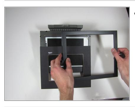
Remove the frame and matte from the device.
