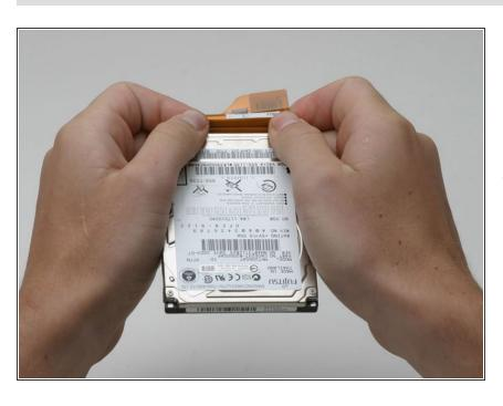
Disconnect the hard drive cable from the hard drive by applying even pressure on both sides while
