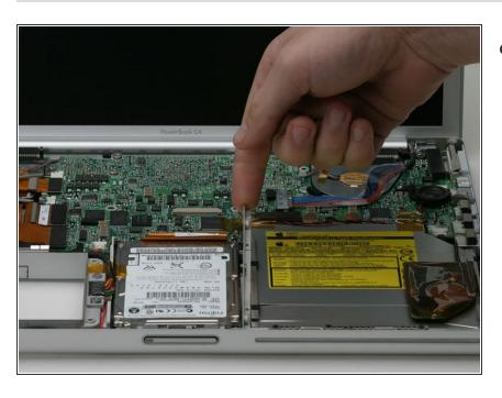
Use a spudger to lift the metal bracket out of the computer.
