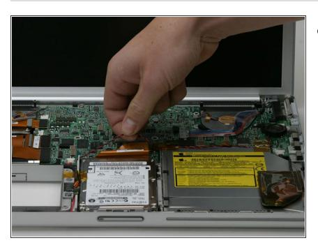
Deroute the red and black speaker cable from under the fold in the hard drive ribbon.
