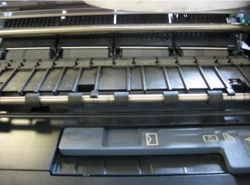
Once you have removed the device top case using the <u>General Device Disassembly Guide</u>, then you can access the rubber paper rollers, located near the front, holding the silver bar in place.
