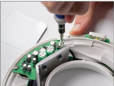
• Remove the three 1 cm T-10 Torx screws.
