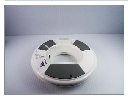
Turn the device upside down so that the three rubber pads are facing up.
