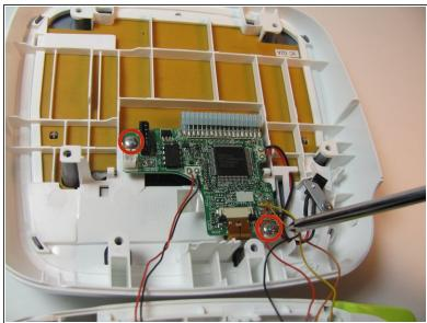
• Remove the two 3/16" screws from the circuit board using the Helping Hand 1/4" screwdriver.
