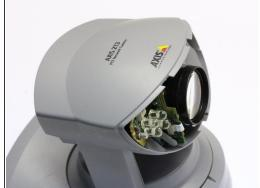
• Take out the screw under the lens. Gently tilt front upwards and remove.
