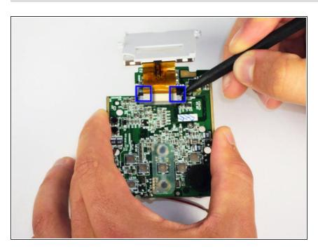
Flip over the circuit board and unlock the two black tabs on the ribbon connector by sliding them upwards.
