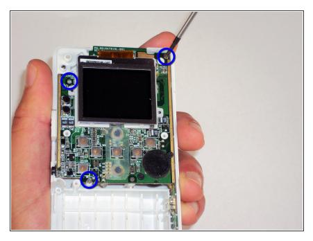
Remove the 3 5mm screws securing the circuit board to the front shell with the #00 Phillips screwdriver.
