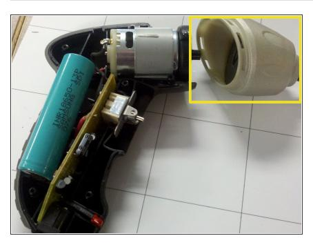
Slide the bit chuck assembly out from the casing half.
