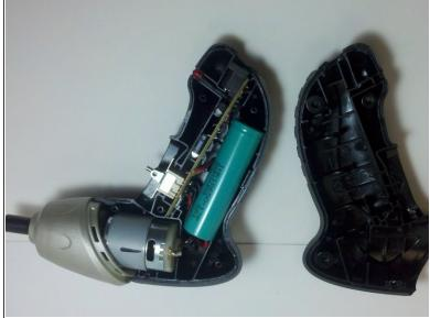
Separate the screwdriver casing halves with the plastic opening tool.
