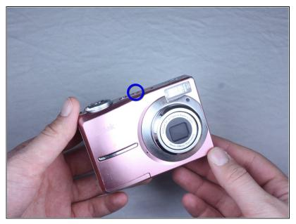
• Turn off camera by firmly pressing the power button that is located on the top of the camera near the selector dial.
