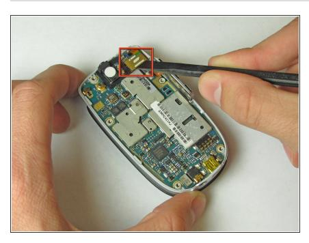
Use the Spudger to detach the screen wire from the logic board.
