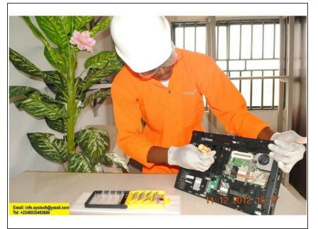
Unscrewing of Hp 625 Keyboard, (6 Screws Noted By Keyboard icon).
