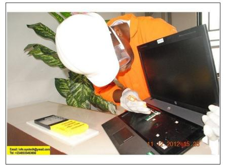
Disconnecting of Hp 625 Power Flex Cable From Connector, ( Fairly Unlock The Locking Mechanism).
