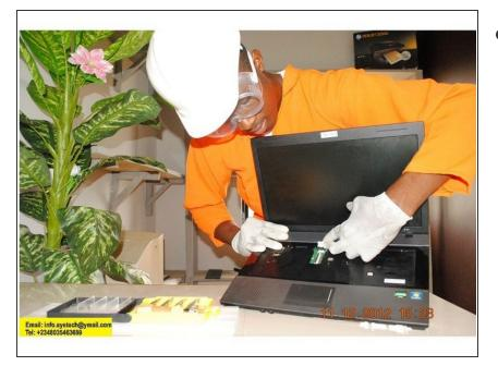
Hp 625 Power Flex Cable Disconnected.
