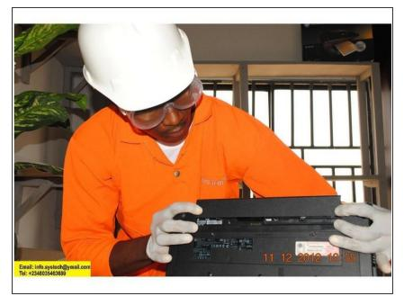
• Removing of Hp 625 Battery.
