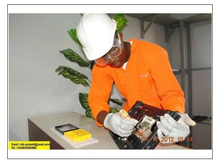
• Unscrewing of Hp 625 Thermal Conductive Heatsink, (6 Screws).
