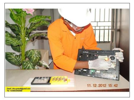
• Unscrewing of Hp 625 Thermal Fan, (1 Screw).
