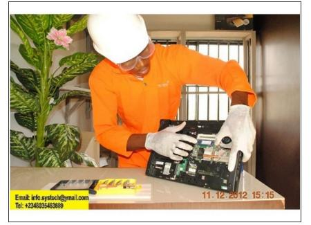
Removing of Hp 625 DDR3 RAM, (Together With Two Hands Expand The Clips a little).
