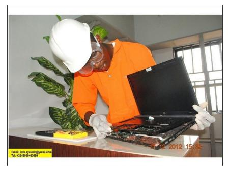
Removing of Hp 625 Front Casein, (Firmly Pry the Casein, Starting from Any Edge).
