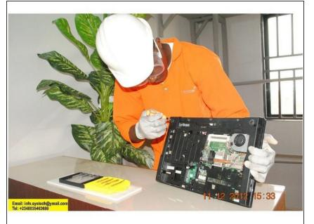
Unscrewing of Hp 625 System Casein, (16 or More Additional Screws Verify Very Well For Additional Screws Needed To Be Unscrewed Before Removing The Casein).
