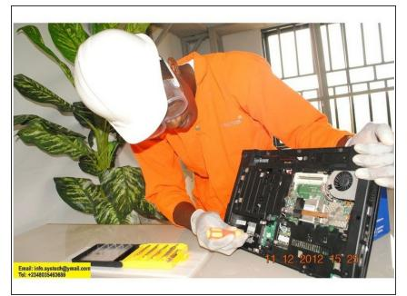
• Unlocking of Hp 625 Palm Rest, Through The HDD Bay.
