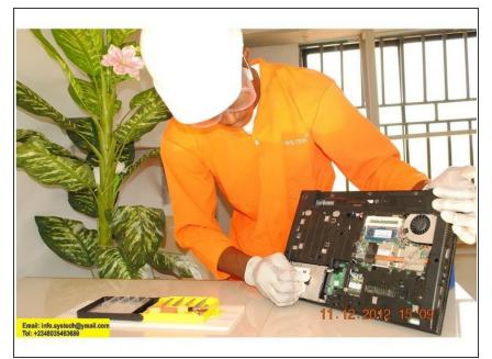
• Removing of Hp 625 HDD, (Gently Slide).
