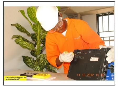
• Unscrewing Hp 625 Service Door (4 Screws).
