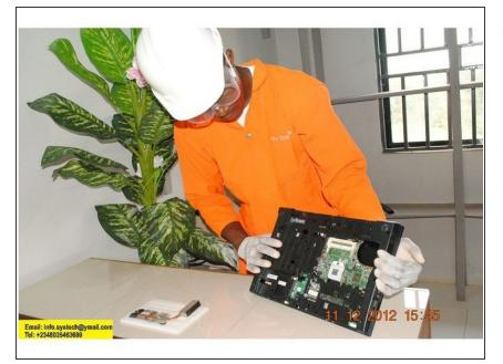
• Hp 625 Thermal Conductive Heatsink Removed.
