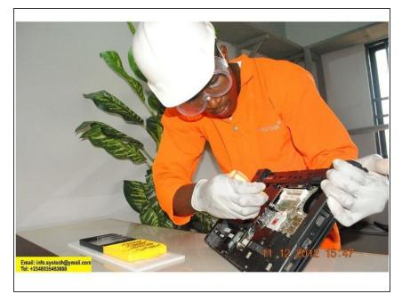
Unlocking of Hp 625 AMD Processor From Socket, (Anti-Clockwise).
