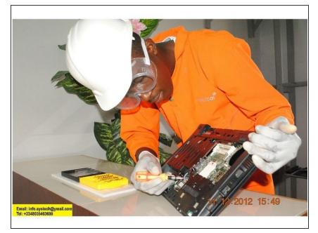
• Disconnecting of Hp 625 Wi-Fi Cables From Wireless Card.
