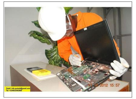
• Disconnecting All Cables of Hp 625 Connected To Motherboard.
