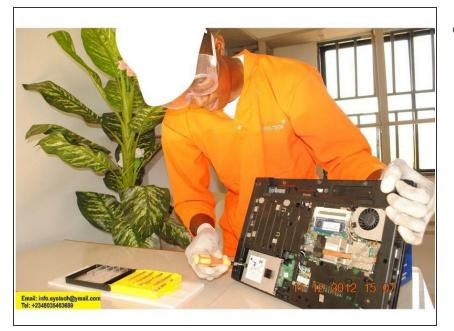
Unscrewing Hp 625 HDD, (3 Screws).
