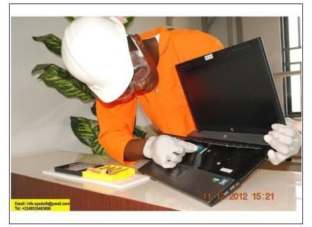
Removing of Hp 625 Keyboard Flex Cable, (Gently Release The Locking Mechanism).
