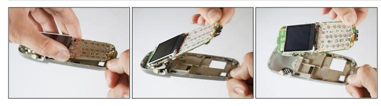
• Gently remove the logic board and LCD screen from the back cover of the phone.
