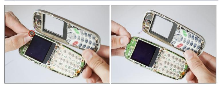
• Using your nails, <u>tweezers</u>, or any precise grabbing tool, pinch the antenna wire connector (clear plastic plug) and pull gently. It should pop out rather easily.
