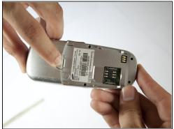
Remove the battery by pressing down on the battery release button while sliding the battery downwards.
