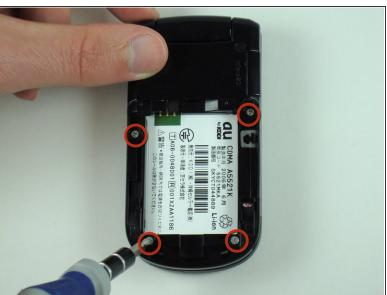
Remove the four screws with the Y0 screwdriver.
