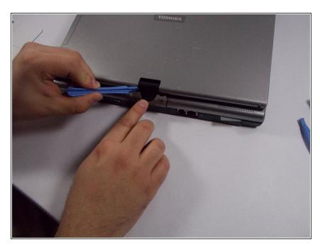
Using the plastic opening tool, remove the plastic hinge cover on the back of the laptop. Use caution not to damage this plastic cover.
