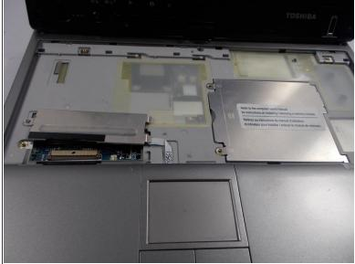
• Use a small phillips screwdriver to remove both metal shields as depicted.
