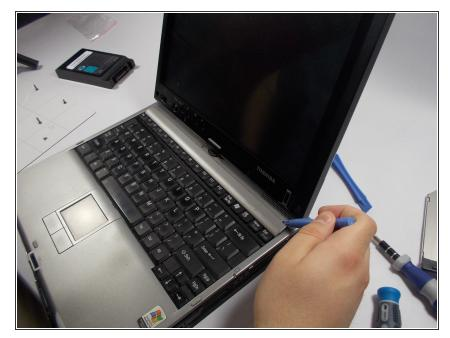
Using the plastic opening tool, remove the plastic cover directly above the keyboard. Make sure to start from the corners of the plastic cover.
