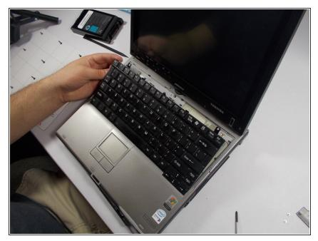
Remove the keyboard, make sure you gently remove any ribbon cables holding it to the rest of the computer.
