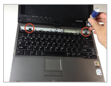
Using the #1 Phillips head screwdriver, remove the two 3.8mm screws.
