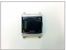
Unscrew the four screws at the back of the watch, then gently use the spudger to open it
