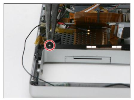
• Remove the nut from the screw just in front of the left speaker.
