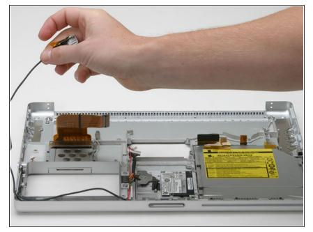
• Deroute the RJ-11 board cable from along the edge of the case.
