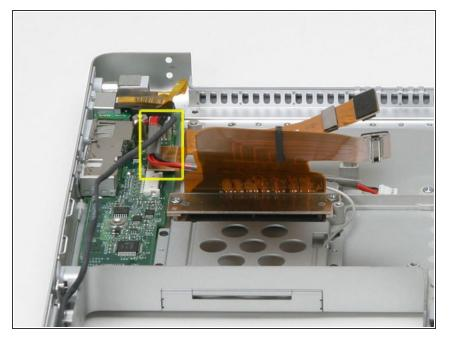
Disconnect the 4-pin power cable and orange ribbon from the DC/Sound card.
