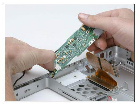
• Disconnect the Bluetooth cable from the DC/Sound card, removing tape as necessary.
