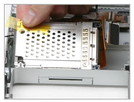
• Lift the PC card cage up from the front, and remove it from the computer.
