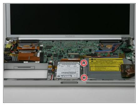
Remove the two 6 mm long silver Phillips screws from the metal bracket to the right of the hard drive, removing tape as necessary.
