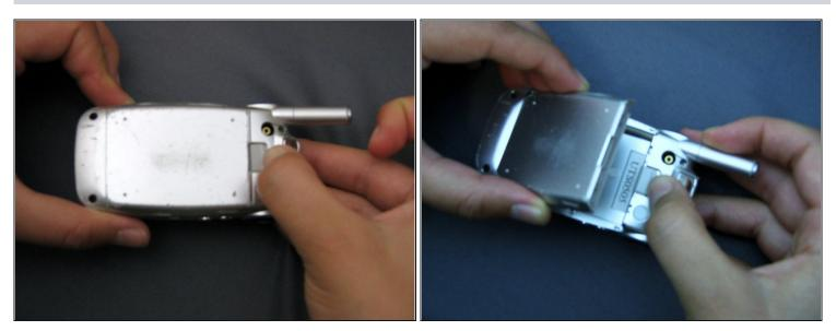
• Hold the phone in one hand, slide the latch up, and pull the battery up to remove it.
