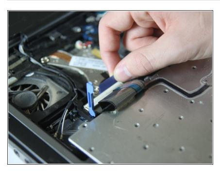
Pull up on the metal bar connected to the socket to detach the ribbon cable
