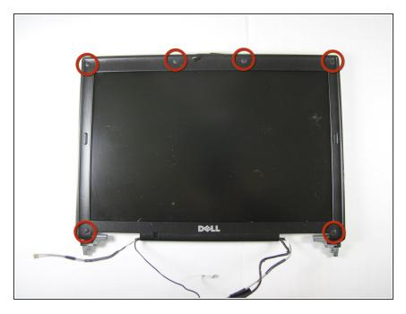
Remove the circular rubber pads as outlined in the picture using a spudger
