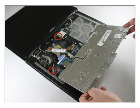
Detach cables that connect the display to the body of the laptop
