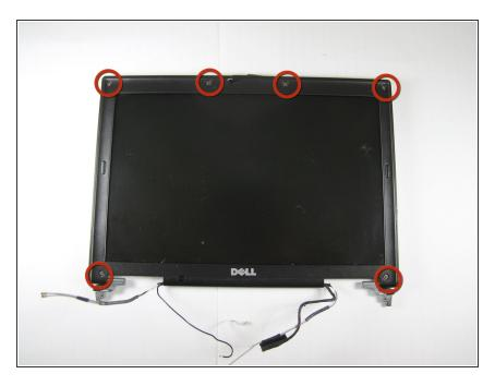
Unscrew the screws that were under the rubber circles using the #00 screwdriver
