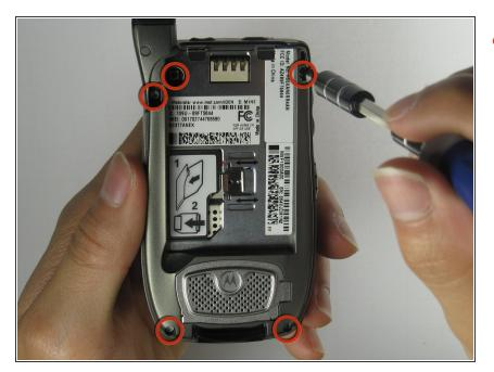
Once battery is removed, untighten the screws located near the edges of the device with a Phillips #00 Screwdriver.
