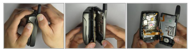
• Grip the device firmly with both hands and carefully open the device.
