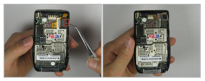
• Carefully grip the side of the hardware attachment with a tweezer and detach from device.
