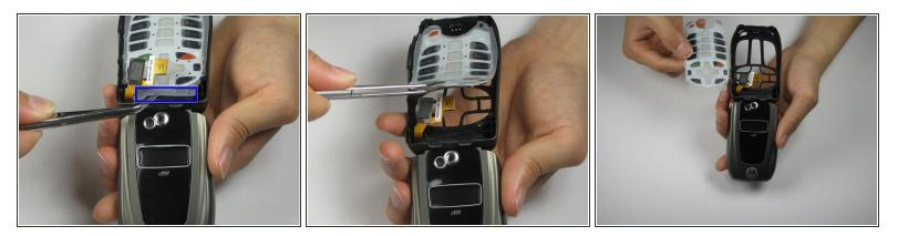
• Carefully remove the keypad by griping on the side of the plastic with a tweezer.
