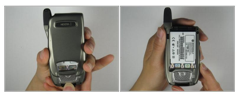
• Slide the back cover towards the antenna while lifting the cover away from the phone.
