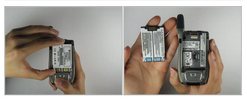
• Lift the battery out of the phone while pushing it towards the antenna.
