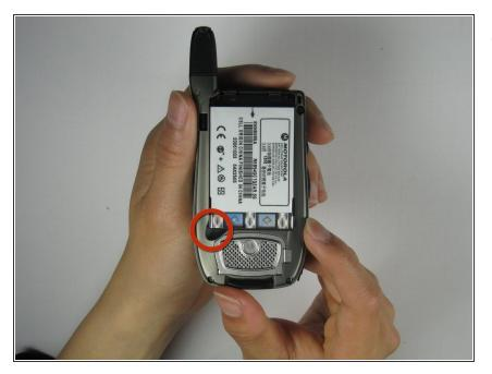
Place your thumb on the indicated corner while stabilizing the phone and the upper portion of the battery with your forefinger.
