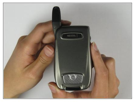
• Use your thumb to slide the back cover locker away from the antenna.
