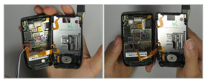
• Carefully remove the hardware by gripping the side of the hardware attachment with a tweezer.
