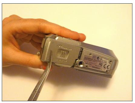
Press and slide the battery cover retainer clip to the left.
