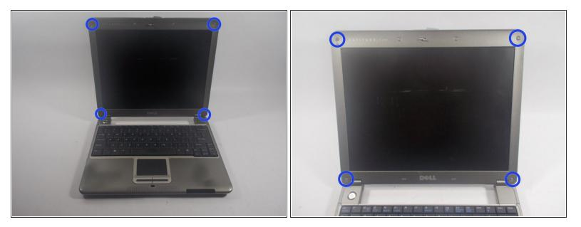
(i) Remove rubber caps on each corner of the front screen with a pinch.
