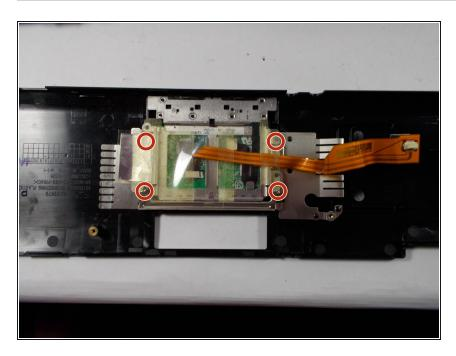
Align the new trackpad so the screw holes line up with their insertion points. Replace the screws with the screwdriver.
