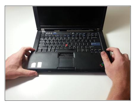
With the screws removed, the trackpad panel should lift as shown.
