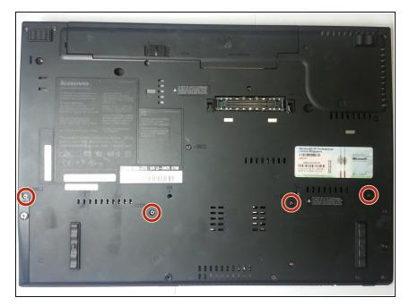
Flip your computer over and remove the four indicated screws with the Phillips #1 screwdriver.
