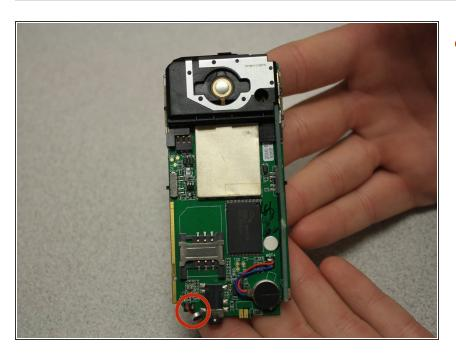
Locate the microphone on the back of the circuit board.
