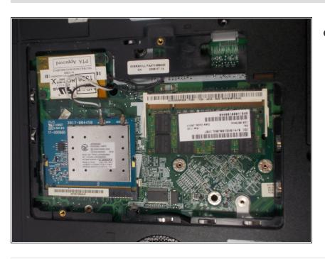
The computer should be open with many of the internal components shown. You can now access the RAM, and wireless card.
