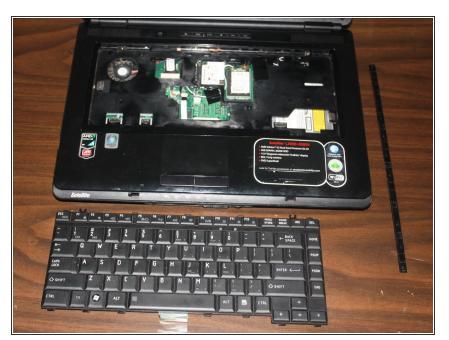
• Remove the keyboard completely from the laptop.
