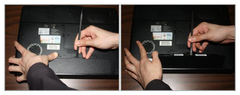
• While holding the left battery lock to the left, lift up the battery using the tab located on the top center of the battery.
