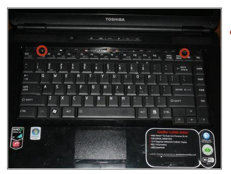
Use a phillips head #0 screwdriver to remove the two 3.75mm screws holding the keyboard in place.
