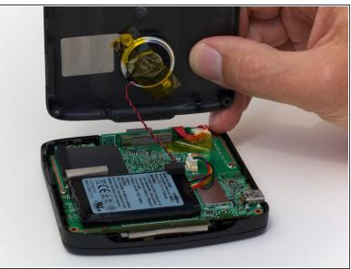
Remove the back cover from the device by separating the back cover along its seam.
