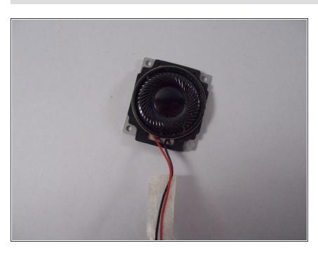
Carefully flip the speaker over and replace or clean the needed parts. To reassemble your device, follow these instructions in reverse order.
