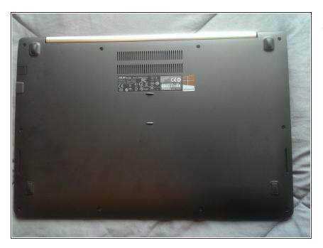
Unscrew the 10 screws on the back cover
