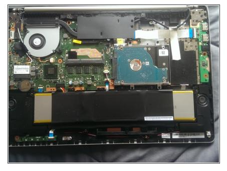
Remove back cover (pry open along the grey/black line, they are held together by clips)
