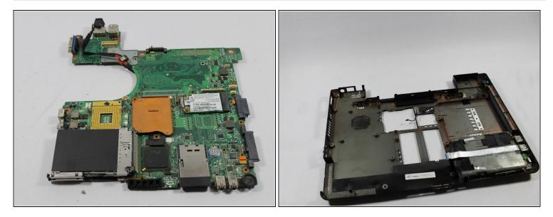
• Lift the motherboard out of the bottom case.
