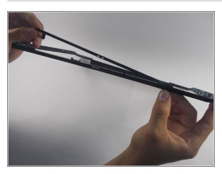
Then connect the latch hook to the latch arm, and test it to make sure it slides over and back into place.
