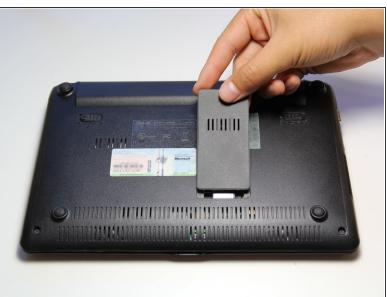
Carefully remove the cover by lifting it with your fingers.
