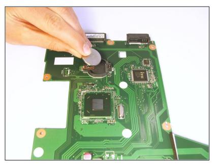
Lastly, lift and remove the CMOS battery from the motherboard.
