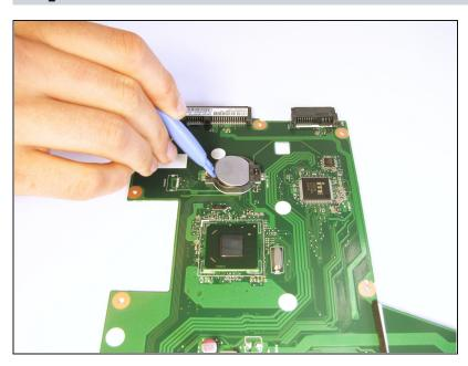
Use the plastic opening tool to pry the battery out of its plastic casing in the motherboard.
