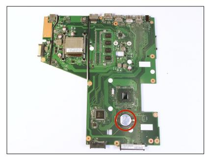
Flip over the motherboard and locate the CMOS battery.
