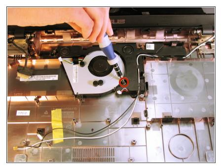
Using the Phillips #0 screwdriver, remove the 5.5 mm Phillips #0 screw holding the fan in place.
