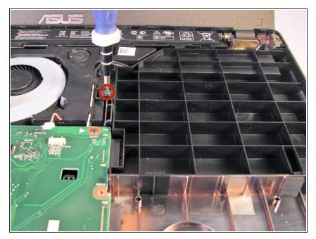
Using the Phillips #0 Screwdriver, unscrew the 5.5 mm Phillips #0 screw that holds the spacer in place.
