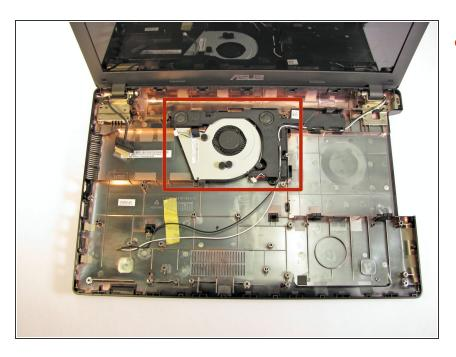
Once the mother board is removed, locate the fan.
