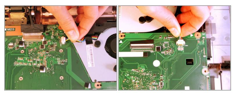
Remove the wires by easily pulling them parallel to the motherboard's surface.
