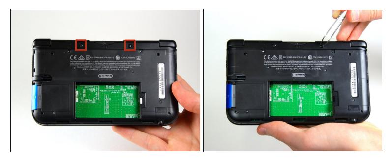
Using tweezers pull out the rubber bumpers that are located at the top of the device on either side of the game cartridge compartment.
