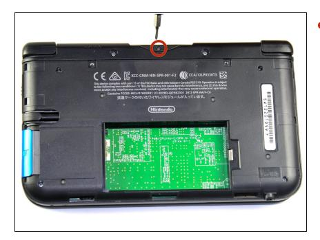
Remove the 2.3 mm screw located above the game cartridge slot with a Phillips #00 screwdriver.
