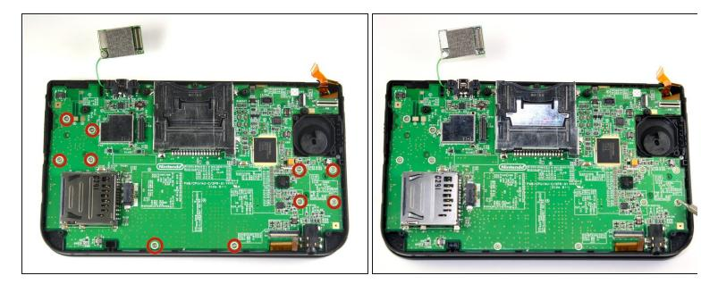
• Remove ten 3.0 mm screws that are located around the face of the motherboard.
