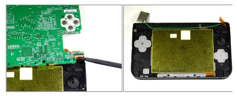
• Using the flat head side of the spudger carefully lift up the flap that attaches the wider ribbon on the upper right side to the motherboard.
