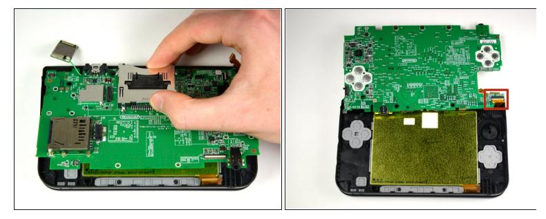
The motherboard will still be attached at the top right hand corner so do not completely detach it at this point.
