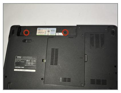
After removing the battery, remove the two screws (3mm Phillips #1) beneath it. These screws hold the Center Control Cover in place.
