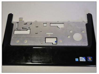
To separate the palm rest from the rest of the computer, use a plastic opening tool to lift up the plastic. It is best to start at one point and work your way around.
