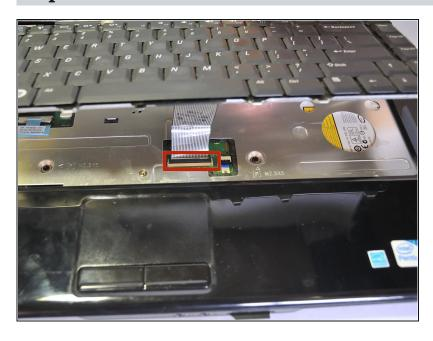
Lift the connector latch that secures the keyboard cable to the connector on the motherboard and remove the cable.
