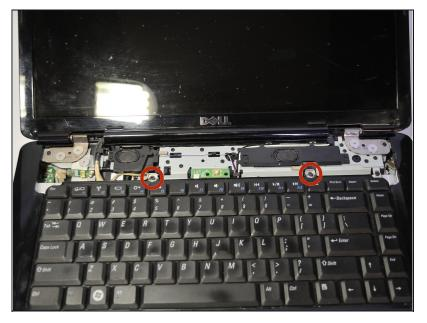
Remove the two screws (5mm Phillips #1) at the top of the keyboard.
