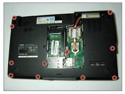
Remove the 11 screws (5mm Phillips #1) from the back of the laptop as marked. One screw is in the middle, by the RAM.
