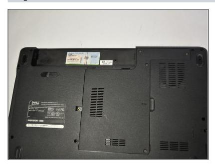
Slide the battery out of the battery bay.
