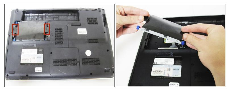
• Pull up on the two plastic flaps on the hard drive enclosure to remove it.
