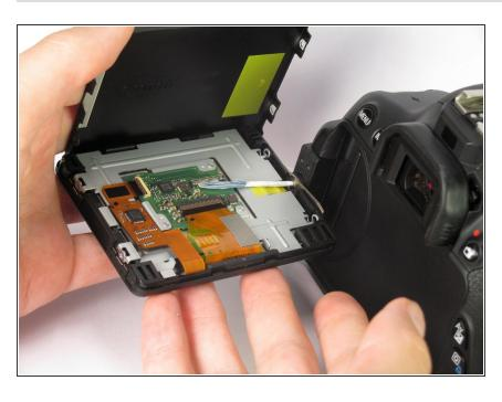
Remove the plastic back of the LCD.
