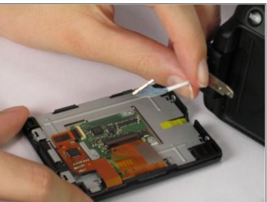
Unplug the blue cable attached to the back of the LCD.
