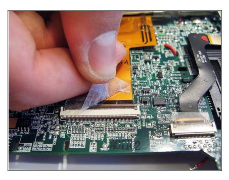
Gently remove the tape covering the yellow ribbon connecting screen to motherboard.
