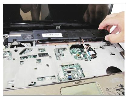
• Remove the speaker assembly from the keyboard tray.
