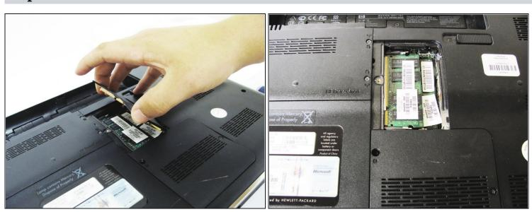
• Remove the RAM cover to reveal the module's underneath.
