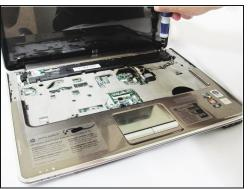
• Locate four 3mm screws in the upper corners of the keyboard tray and remove them using a #00 Phillips screwdriver.
