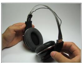
Using the plastic opening tool, gently pry the headband cushion directly away from the plastic portion of the headband as shown. Pry the plastic portion a small amount and then move the opening tool sideways along on the headband. Repeat on both sides until the cushion separates from the top plastic part of the headband.
