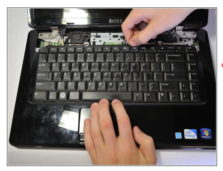
Slide the keyboard out and away from the laptop and lift it up to access the keyboard connector.
