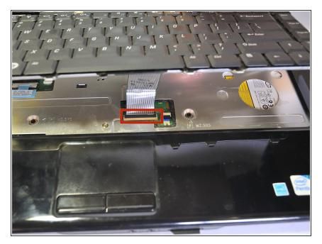
Lift the connector latch that secures the keyboard cable to the connector on the motherboard and remove the cable.
